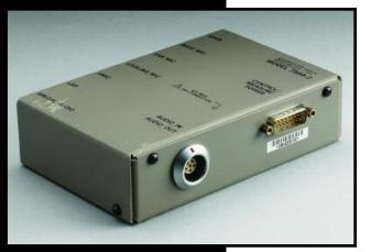
The 7999-2 Three-Pole Audio Multiplexer Module contains a three-pole  $1\times3$  multiplexer, and a 3-pole  $1\times4$  multiplexer for switching audio signals. For minimizing the effects of noise, the input and output connectors are shielded, high quality audio connectors, and the module is enclosed in an aluminum case. In addition, each input and output line has an RF filter for filtering out high frequency noise.
